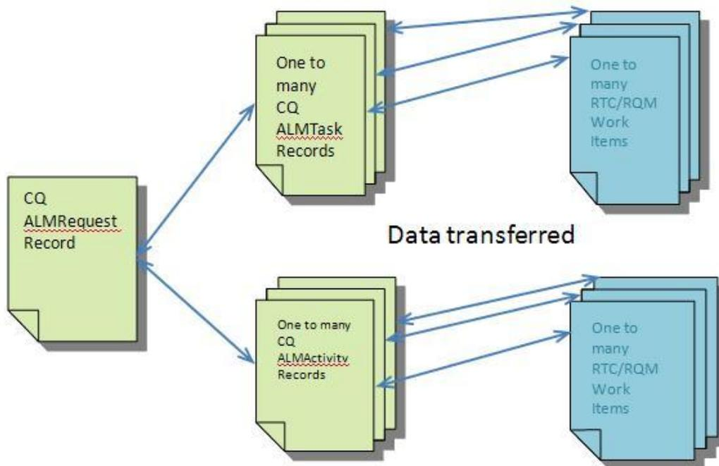
Figure 7. CQALM connected with Rational Team Concert/Rational Quality Manager using ClearQuest Connector.
